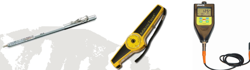
From left to right: pen style magnetic pull-off gauge; banana style magnetic pull-off gauge; digital magnetic induction gauge.
